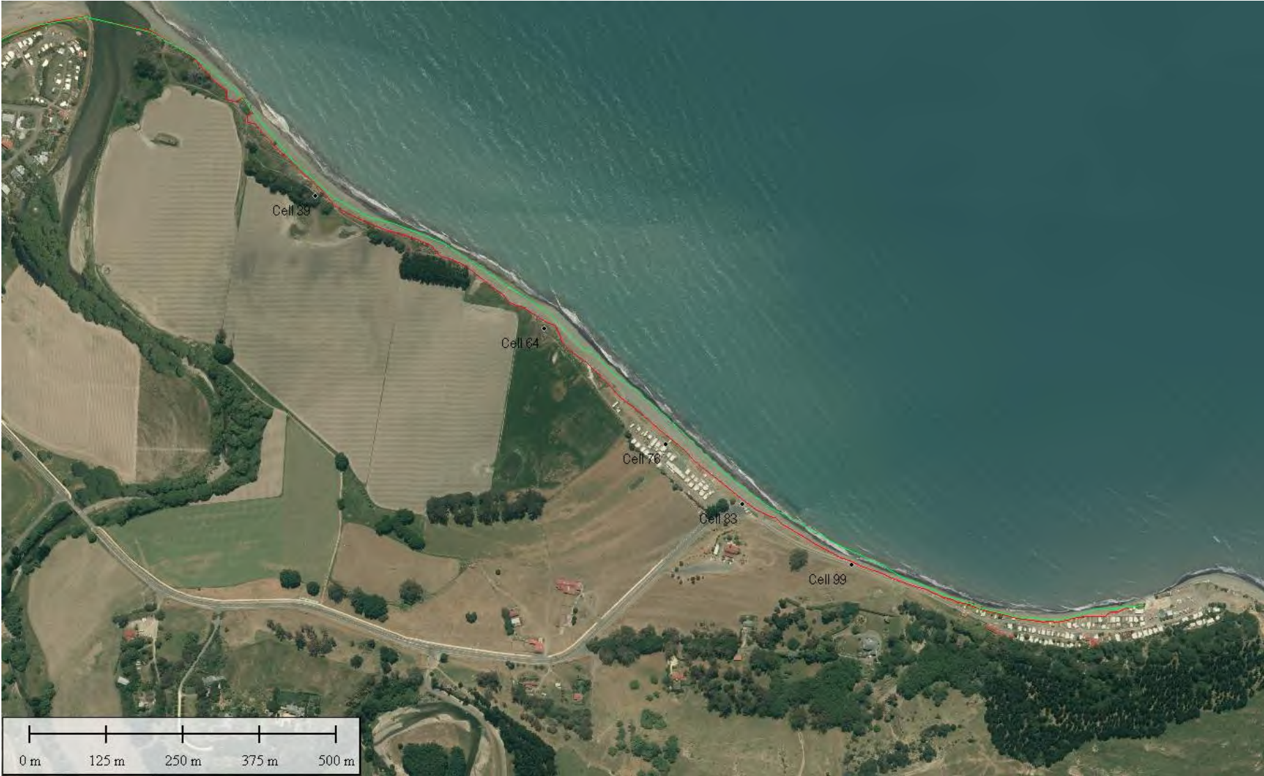
Figure 3.5: Historical shoreline movement – Base photograph 2009, 1980 vegetation line (red) and 2009 vegetation line (green)
