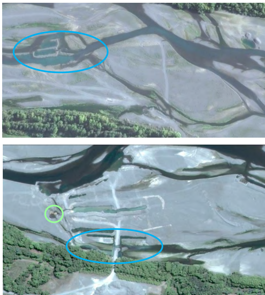
Figure 4. Aerial imagery of a gravel extraction site in the Ngaruroro River downstream of Maraekakaho during 2015 (top) and 2016 (bottom). Note turbidity plumes in side braids (light blue and brown coloured water within blue ovals) indicating elevated levels of suspended fine sediment. Turbidity plumes are associated the bundled gravel areas (top blue oval) and machinery crossing areas (bottom blue oval). Machinery can be seen working under green circle (bottom).
