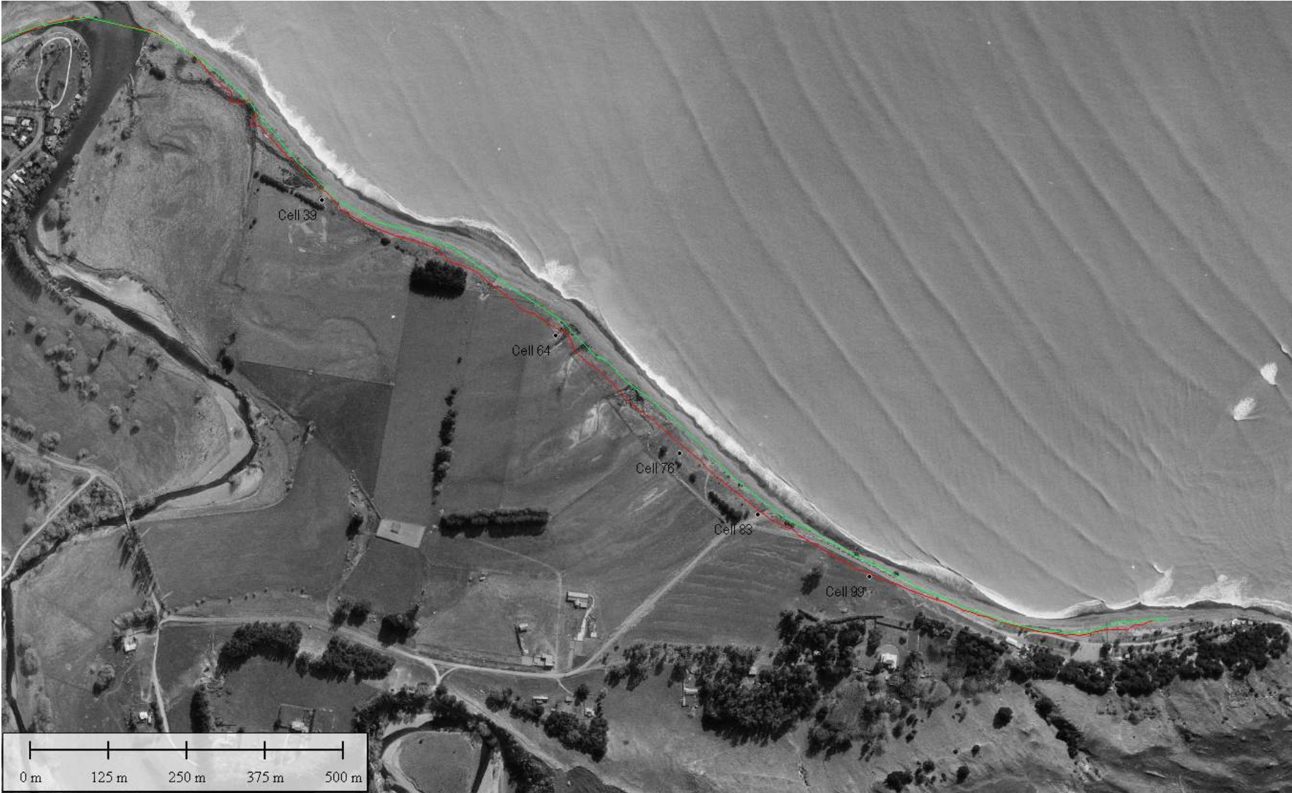
Figure 3.4: Historical shoreline movement – Base photograph 1963, 1980 vegetation line (green) and 2009 vegetation line (red)
