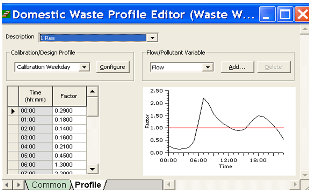
Figure 6- Dry Weather Flow Pattern
