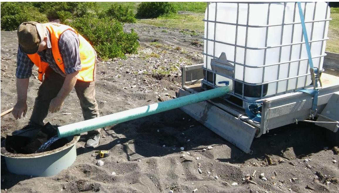
Figure 4 Set up of drainage testing apparatus
