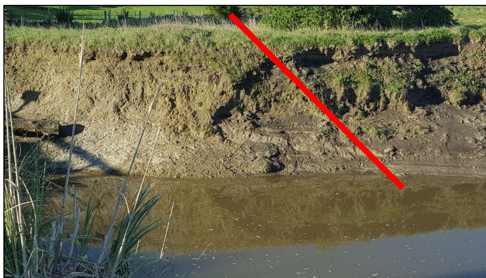
Figure 6.9: The interface between the sedimentary rock (left of red line) and the coastal gravel/sand (right of red line). (Source: H. Lowe)
