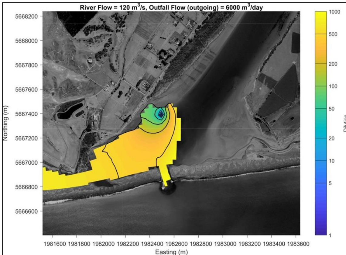
Figure 8.5: Dilution of Future Main WWTP Discharge of 6,000 m 3 /d at 2 x Median River Flow (Source: eCoast, 2018:C1.1)
