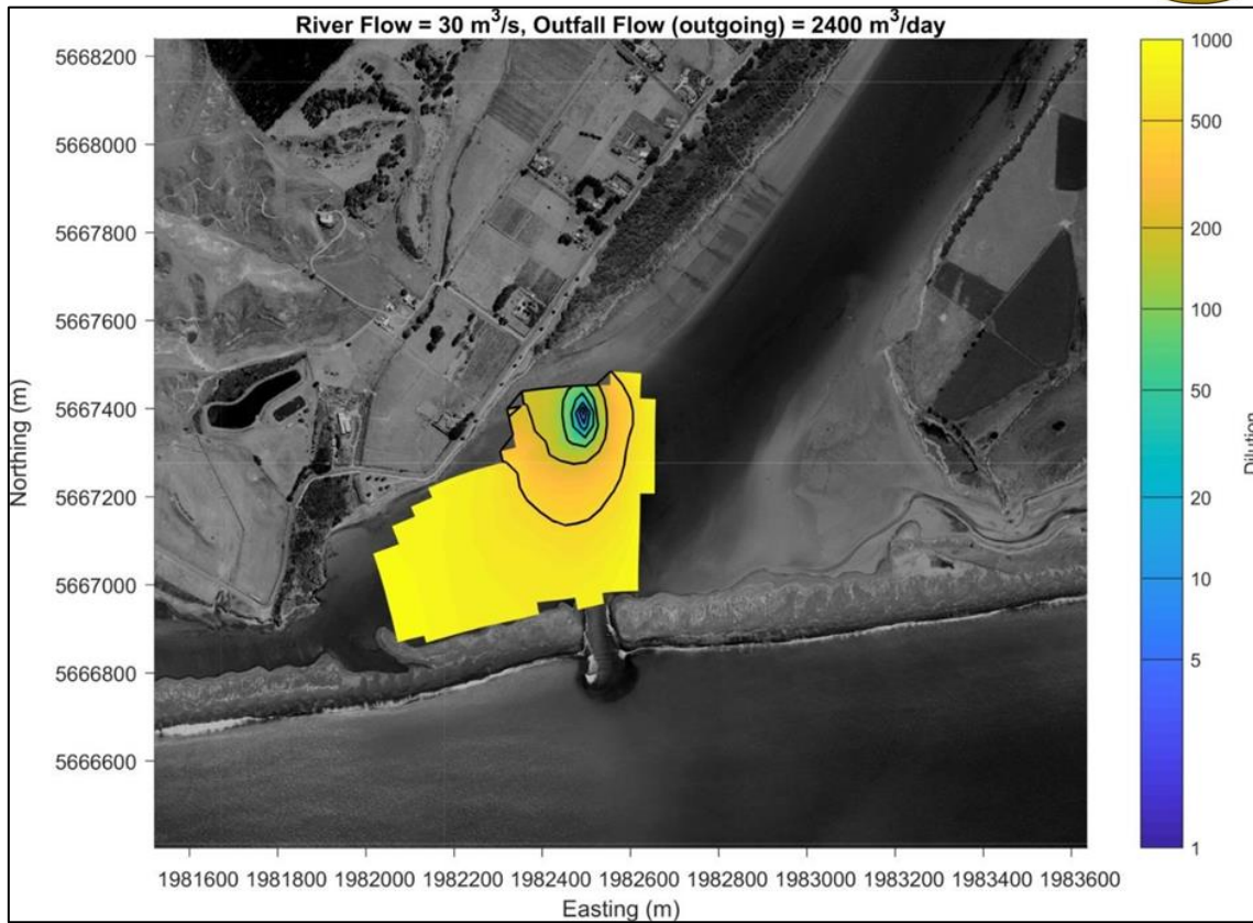
Figure 8.3: Dilution of Future Main WWTP Discharge of 2,400 m 3 /d at ½ Median River Flow (Source: eCoast, 2018:C1.1)
