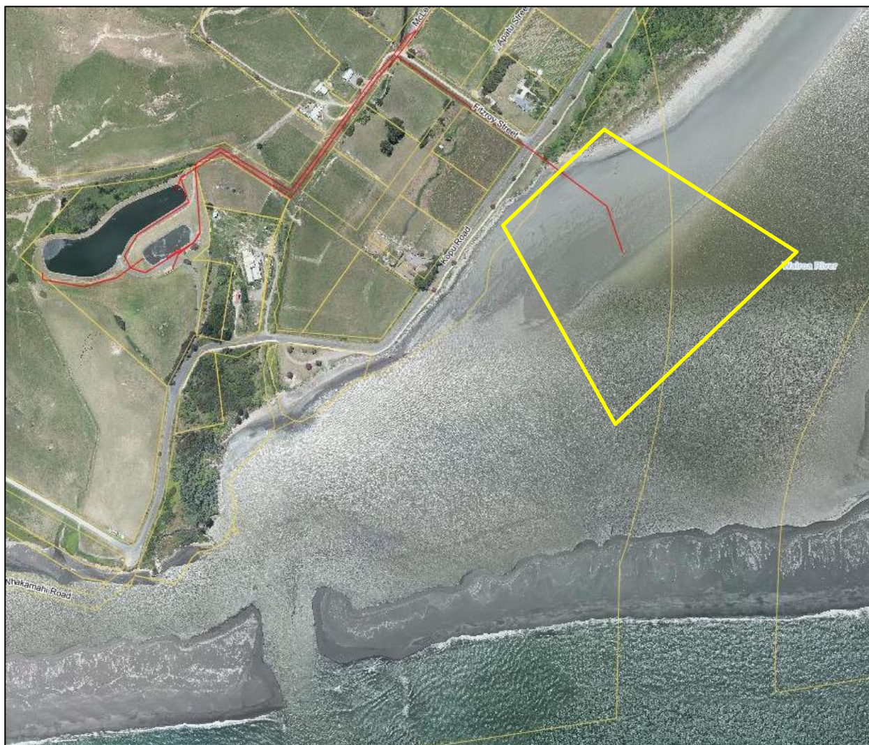
Figure 5.1: Main WWTP Outfall Relocation Area
