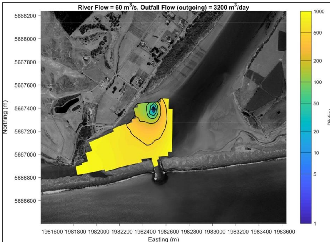
Figure 8.4: Dilution of Future Main WWTP Discharge of 3,200 m 3 /d at Median River Flow (Source: eCoast, 2018:C1.1)
