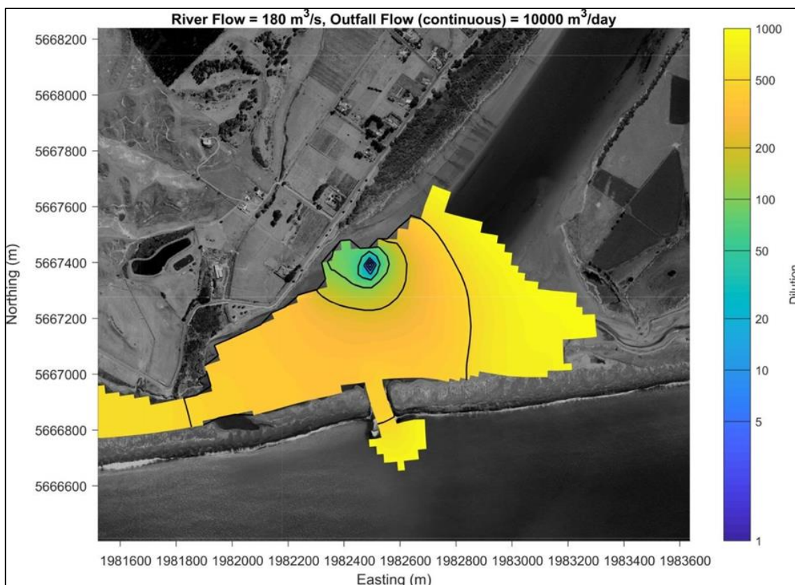
Figure 8.6: Dilution of Future Main WWTP Discharge of 10,000 m 3 /d for 24 hours at 3 x Median River Flow (Source: eCoast, 2018:C1.1)
