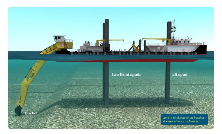
out of the water, a part of the weight of the dredger is now transferred via the spuds to the seabed, resulting in an increase in anchoring. This is sufficient to deliver the required resistance to the digging forces. Secure anchoring makes the BHD less sensitive to waves, currents or the wake of passing vessels.
