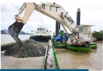
One advantage of a BHD is its ability to dredge a wide range of subsoils, clayey soils, stones, even materials containing boulders or debris.
