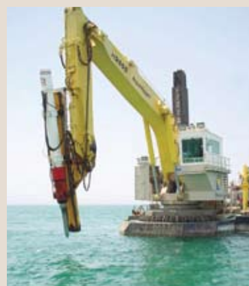
Demag with IHC Hydrohammer® rock breaker
