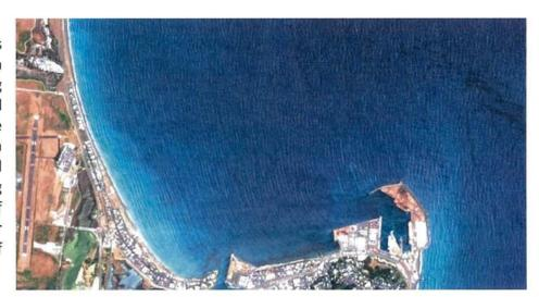
The distortion is caused by the shallower area under the water, created by the dumped sand slowing down the waves relative to the waves either side, that are in deeper water.
