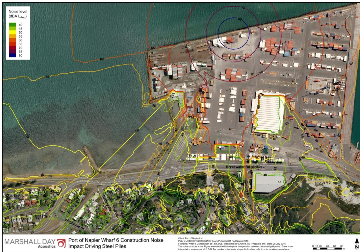
Figure 14-1: Predicted construction noise levels
