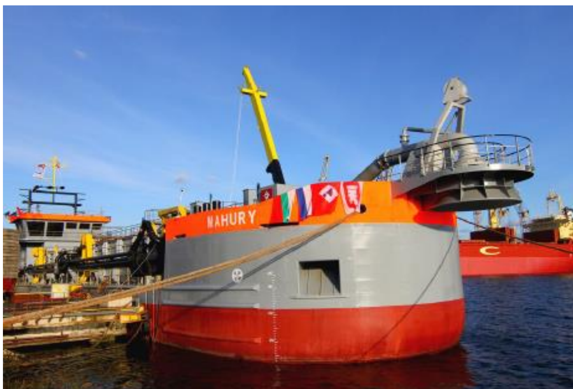
Figure 3-9: Mahury Trailing Suction Hopper Dredge (TSHD)
