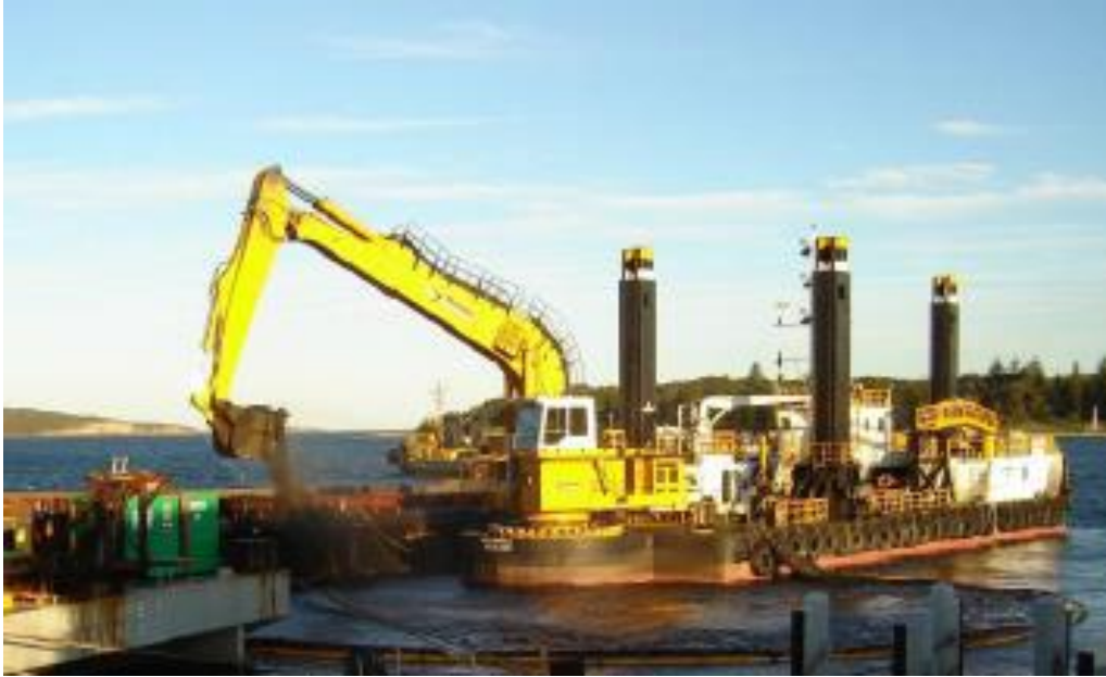
Figure 3-7: Machiavelli Backhoe Dredge (BHD)
