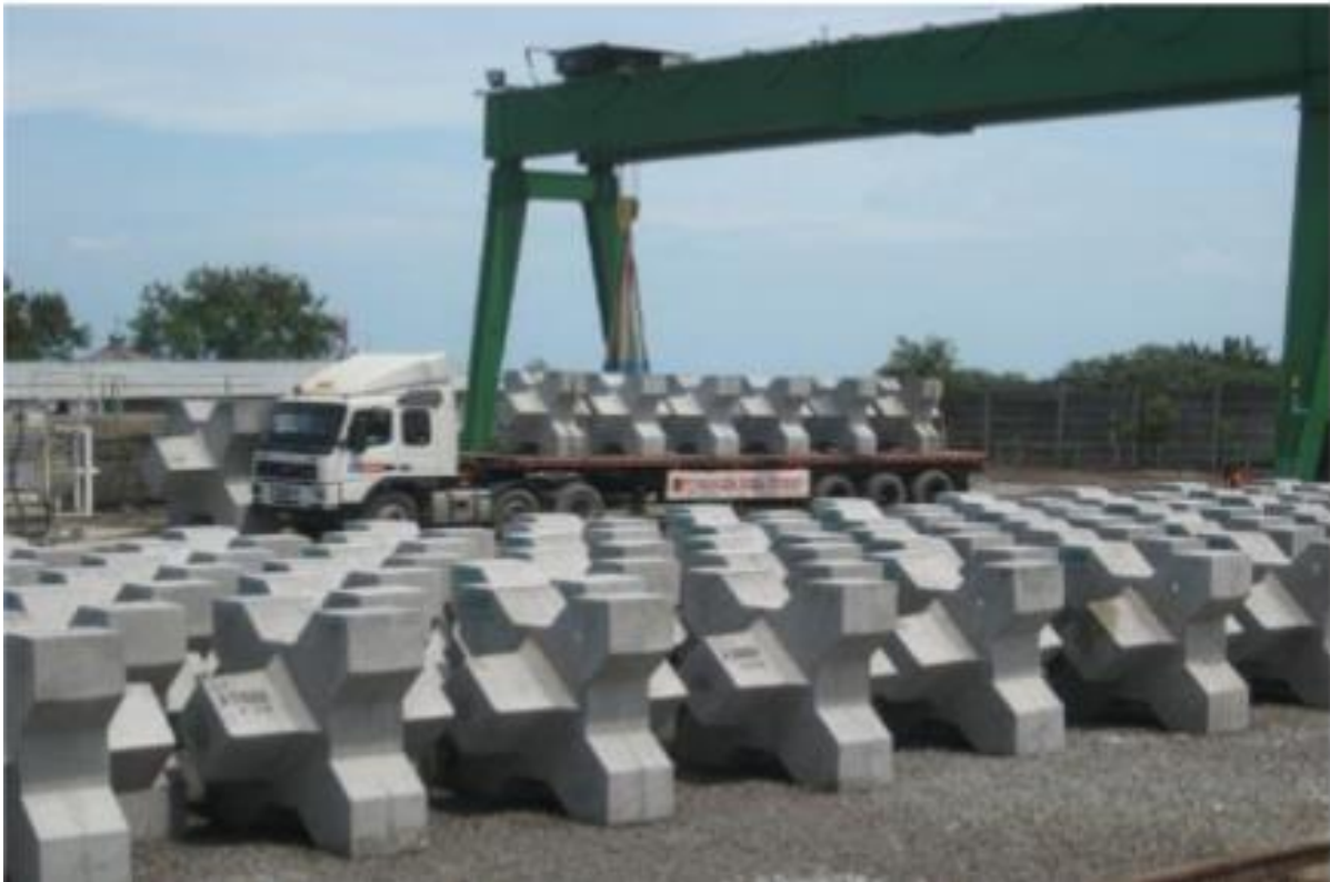
Figure 3-4: Typical revetment armour block units which would be manufactured off-site and transported in
