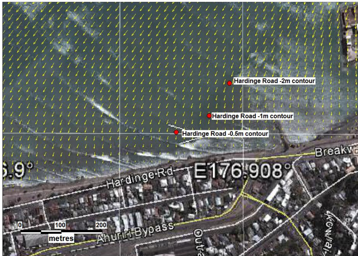
Figure 6-18: Hardinge Road surf break with discrete locations for surfing amenity analysis plotted, and indicative modelled wave approach vectors
