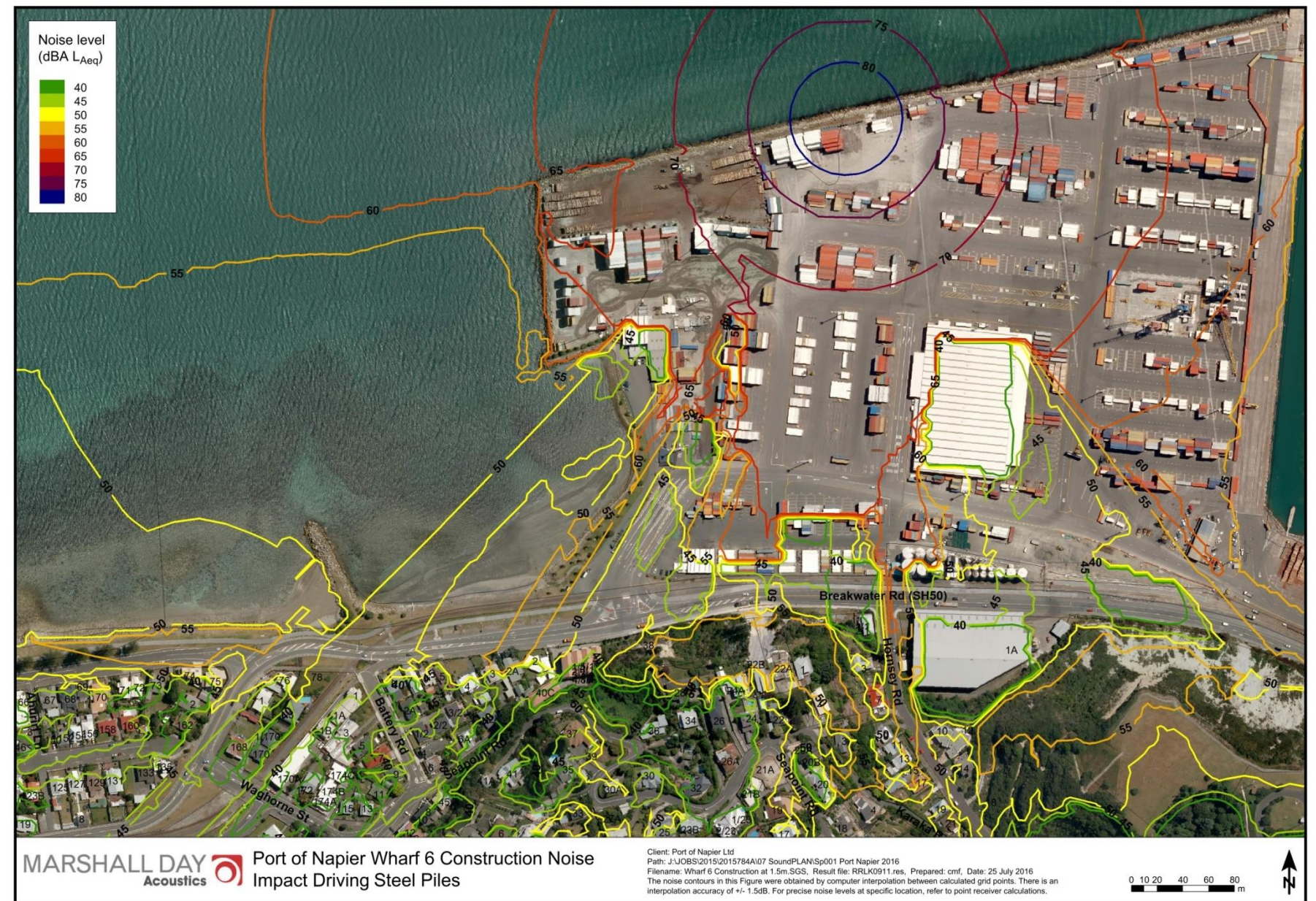
Figure 3: Predicted Noise Levels for Impact Driven Steel Piles
