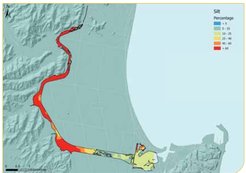
Figure 10-6. Top: Waitangi Estuary in February 2019 following a high flow event. Bottom: The proportion of mud ( <0.063\text{mm} ) in Ahuriri Estuary. Greater than 25% (orange) indicates sediment stress and likely loss of some sensitive species; greater than 60% (red) indicates a high level of sediment stress.
