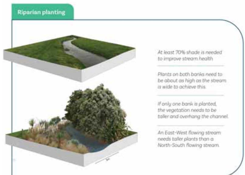
Figure 18-17 Design for effective riparian planting to provide shade and improve stream health.
