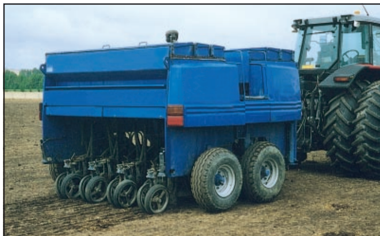
Direct drilling protects top-soil from wind erosion and run-off during heavy rain.
