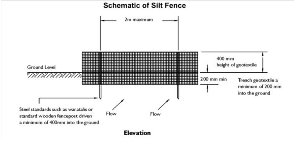
Figure 2: Silt Fence standard detail
