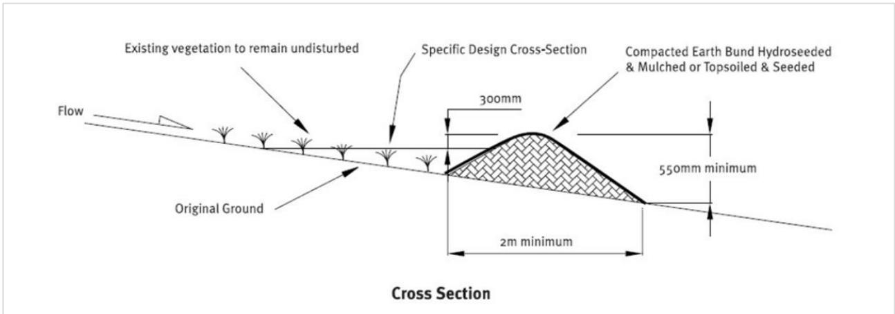
Figure 4: Clean water diversion channel and bund typical detail
