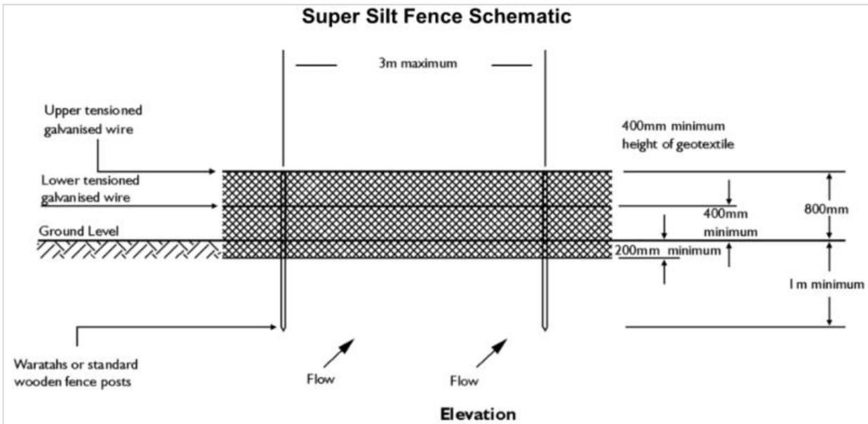
Figure 3: Super Silt Fence standard detail
