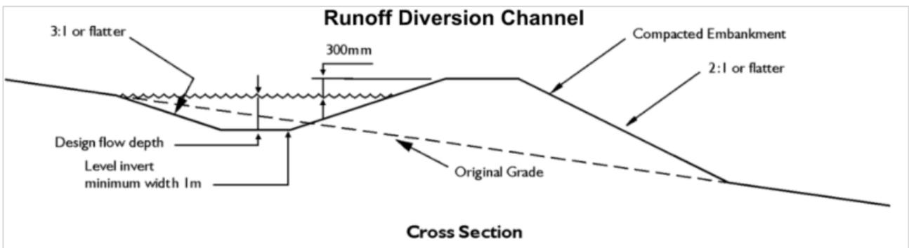
Figure 5: Dirty water diversion channel and bund typical detail
