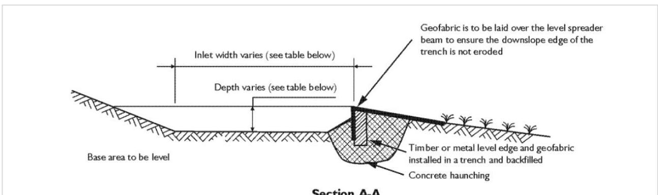
Figure 6: Level spreader cross section
