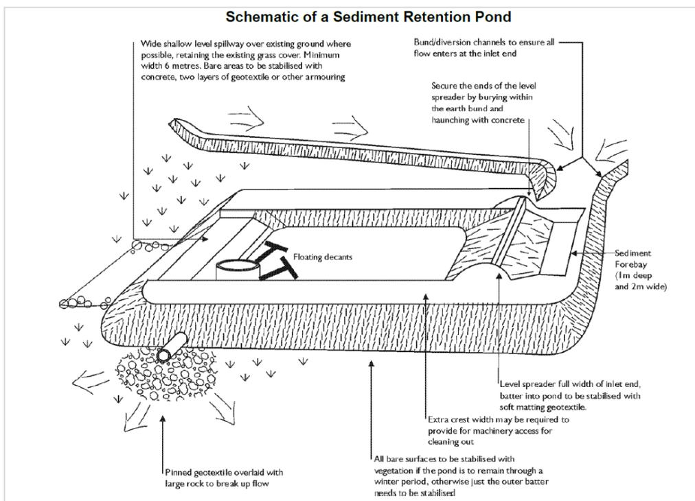
Figure 8: Sediment Retention Pond Schematic (refer to HBRC guidelines Figure 6-1)
