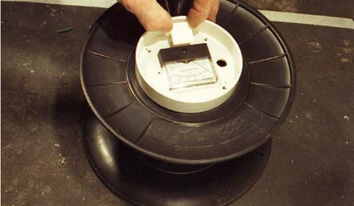
Figure 26. Attach adhesive strip.
