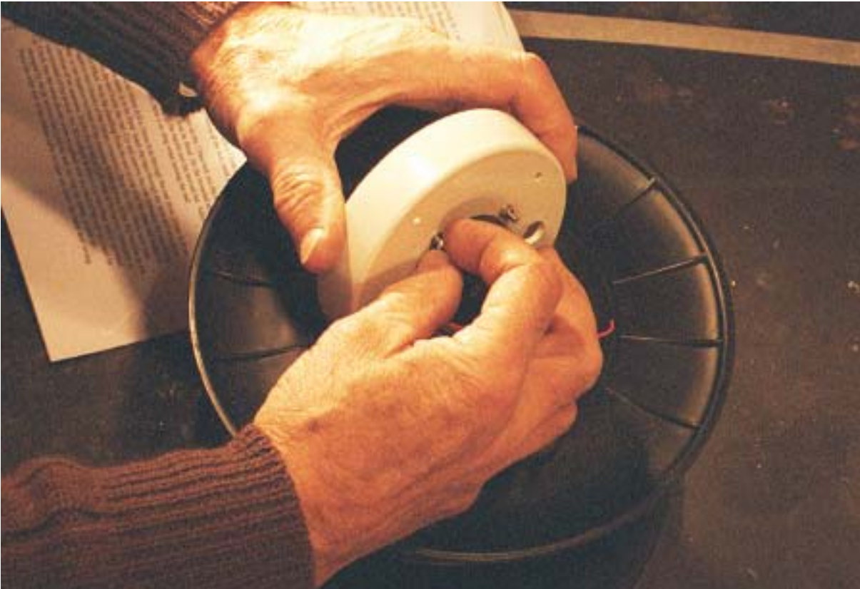
Figure 30. Screws nuts onto meter screws with flat and spring washers.
