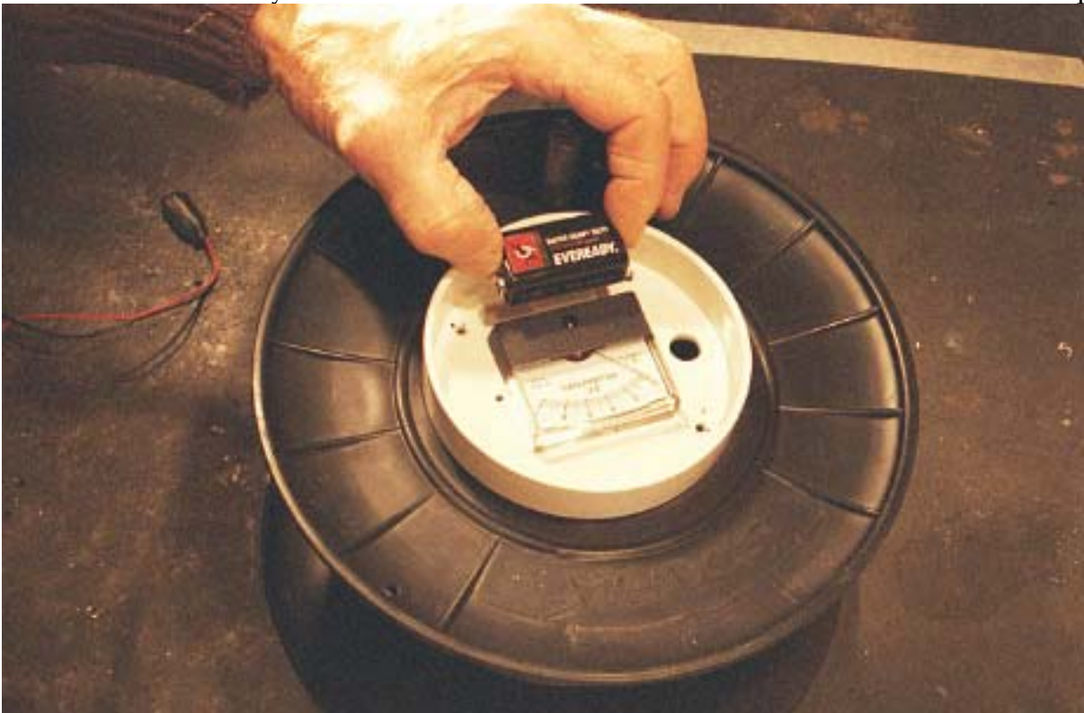
Figure 27. Attach battery to adhesive strip.
