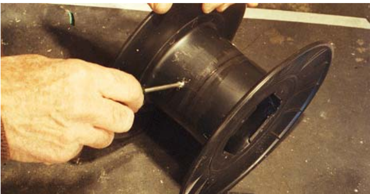
Figure 11. Insert screw into hub and wooden brace.
