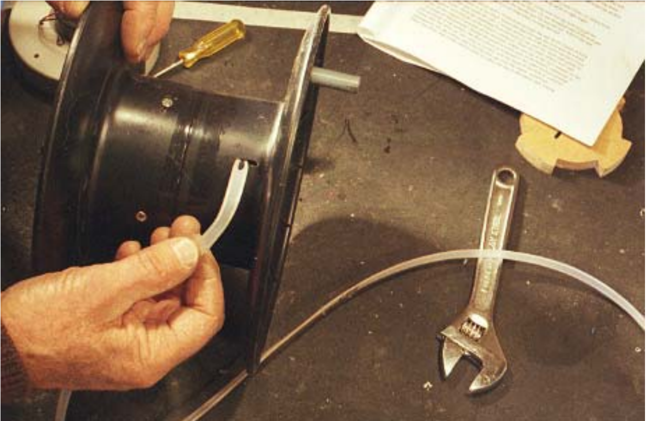
Figure 35. Put antennae ribbon into reel slot.
