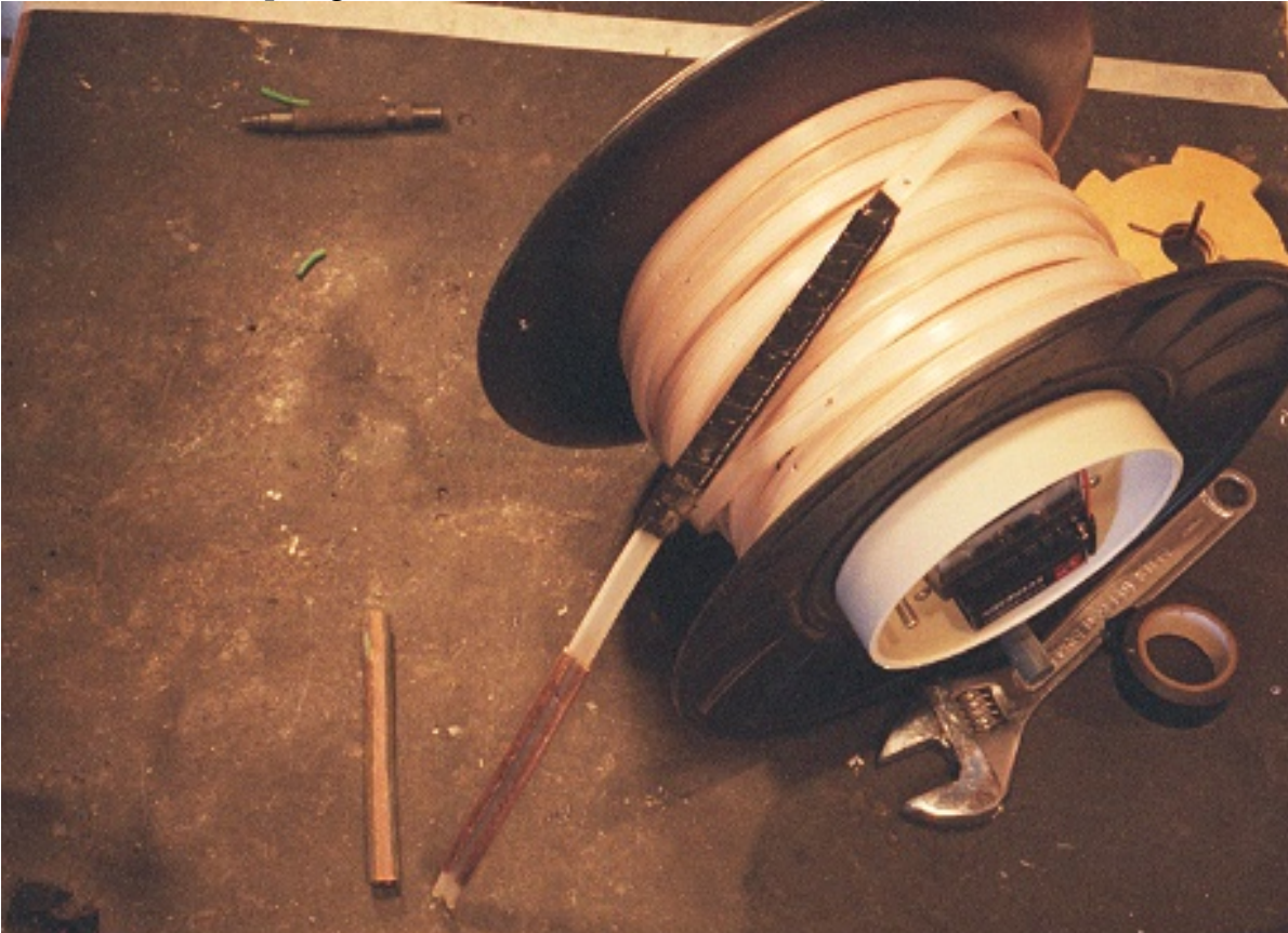
Figure 46. Attach copper sheath to antennae ribbon end.
