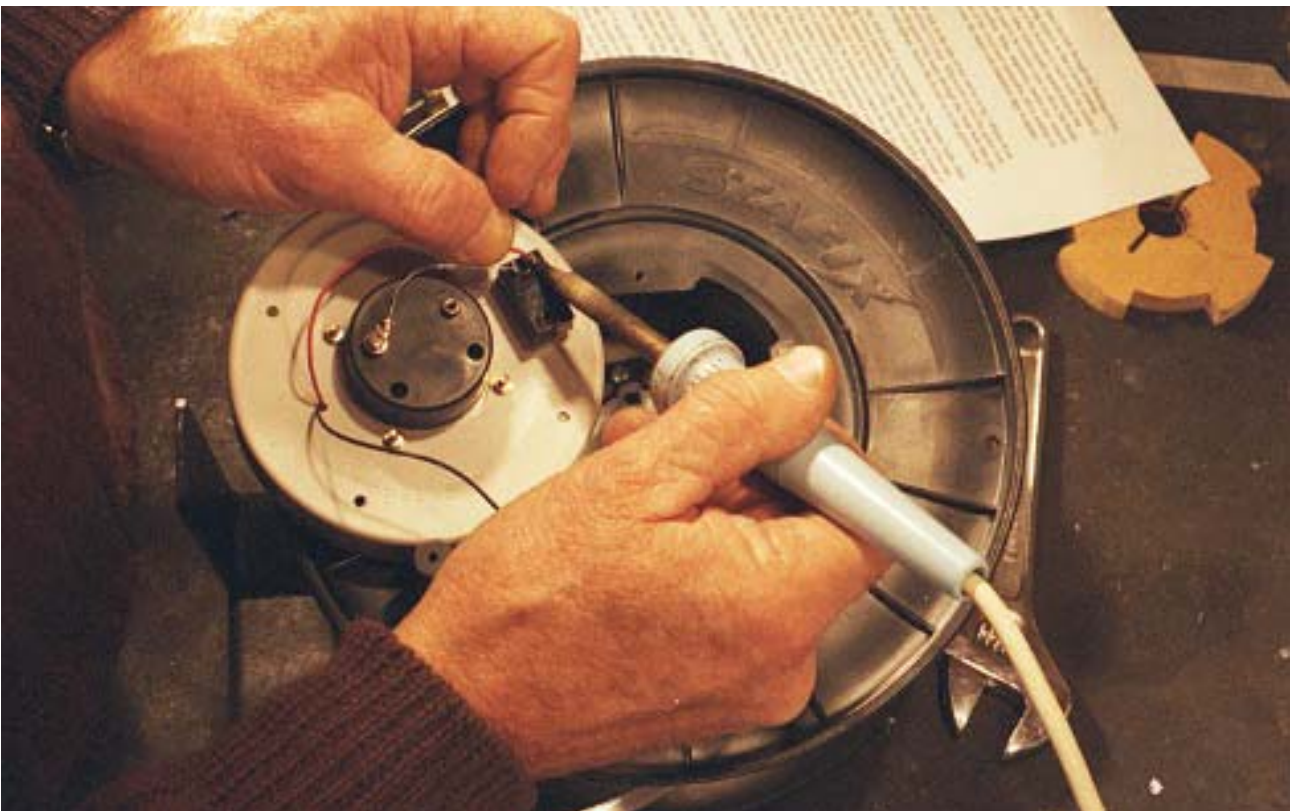
Figure 40. Solder positive (red) battery wire to toggle switch.
