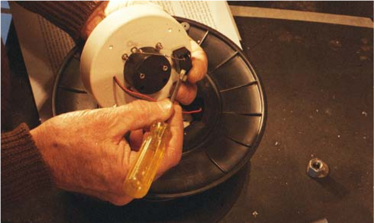
Figure 32. Attach toggle switch.
