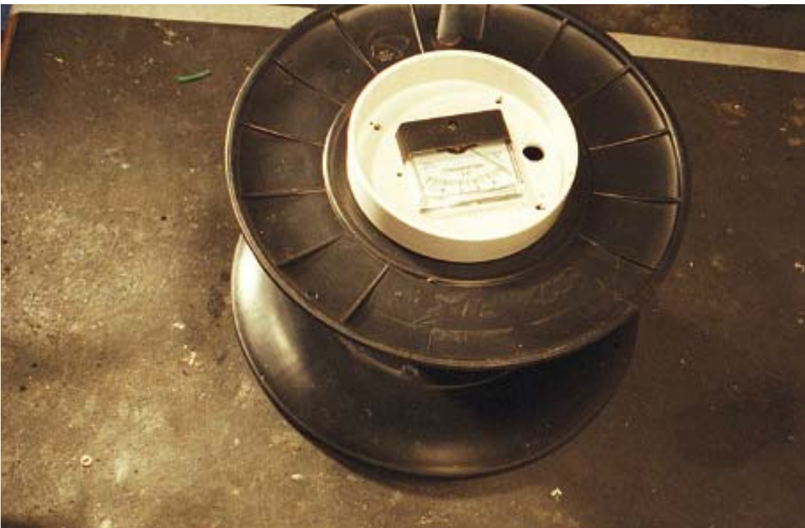
Figure 25. Meter set into cap and reel.
