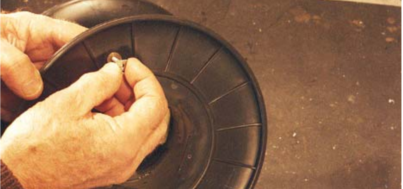
Figure 12. Inserting gutter bolt.
