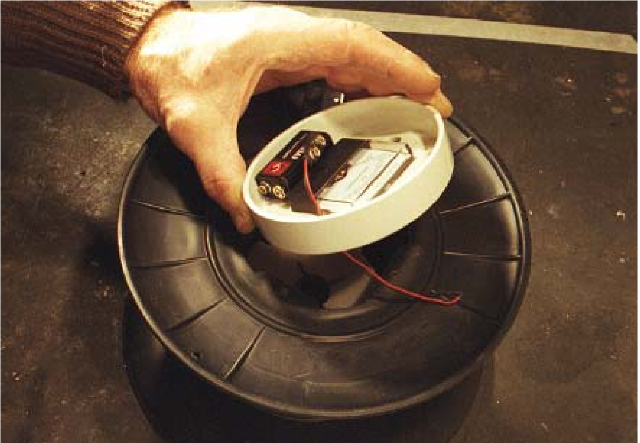
Figure 28. Battery wires through cap hole.
