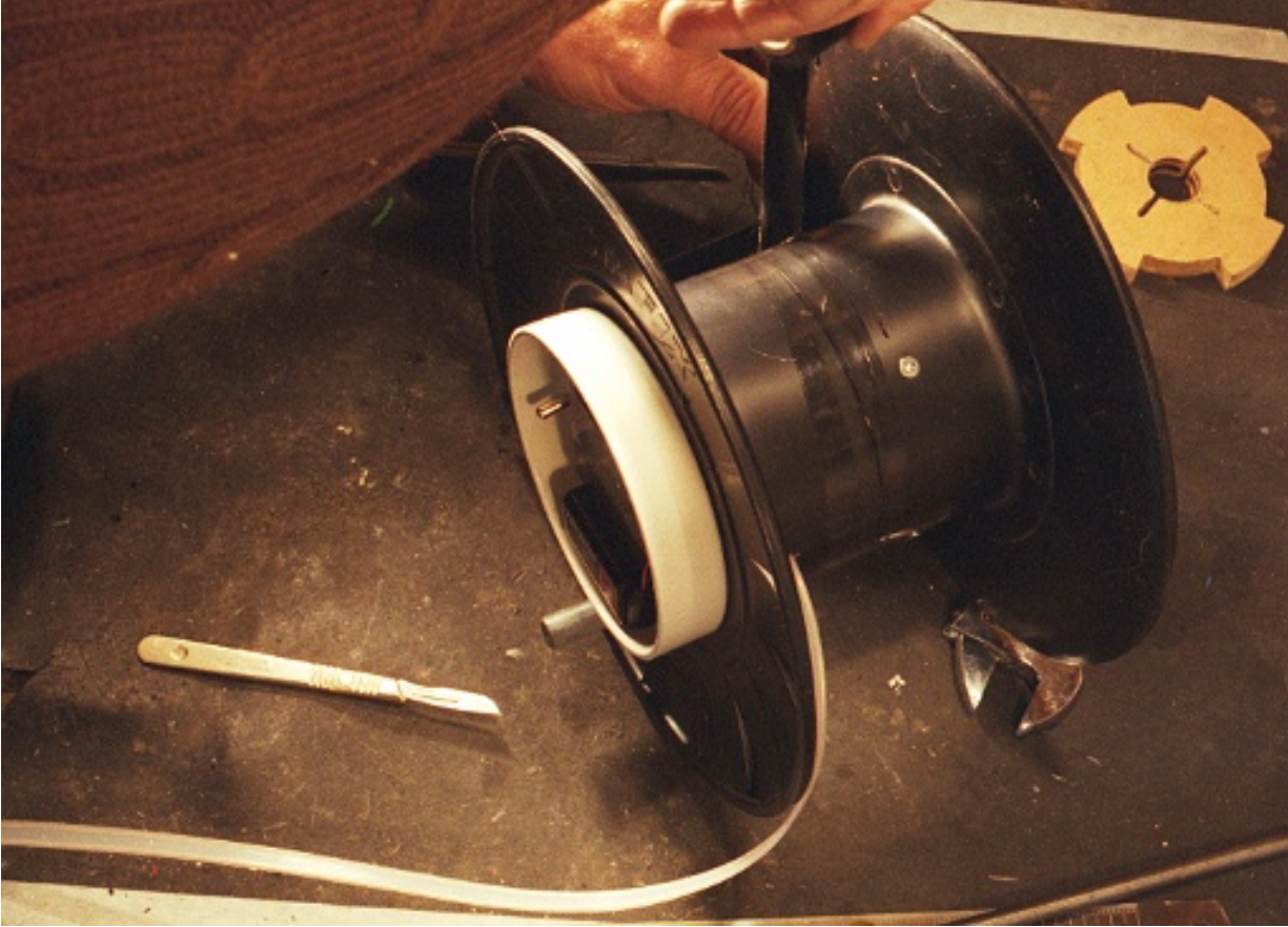
Figure 44. Wrap antennae ribbon around reel hub.
