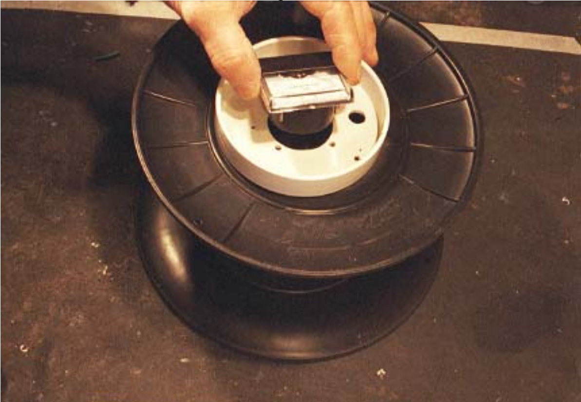
Figure 24. Inserting meter into PVC cap.
