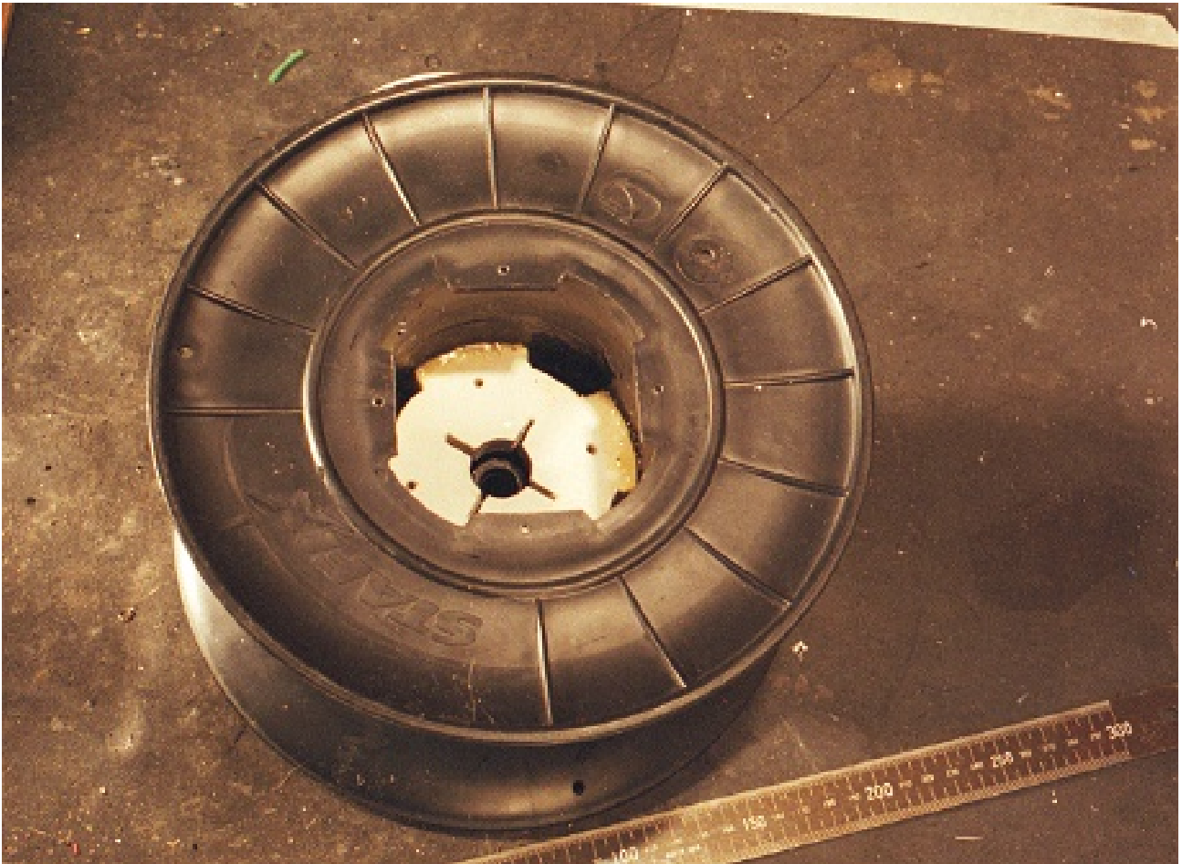
Figure 9. Insert wooden brace into reel hub.
