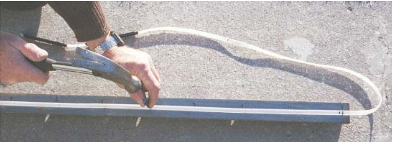
Figure 48. Mark antennae ribbon length increments.
