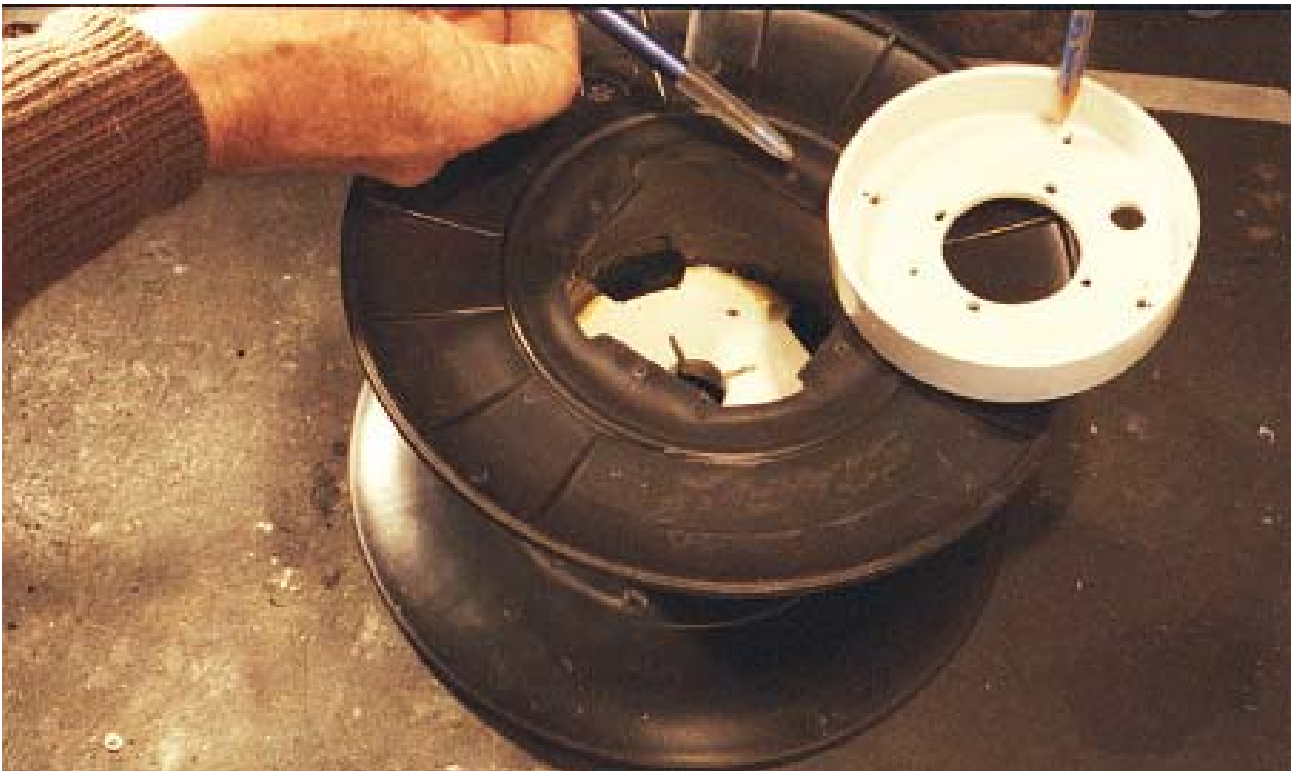
Figure 22. Mark cap and reel for later realignment.
