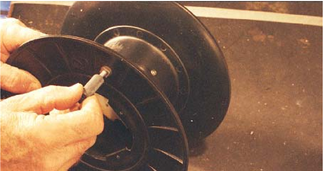
Figure 13. Screw on the tapped wooden dowel handle.
