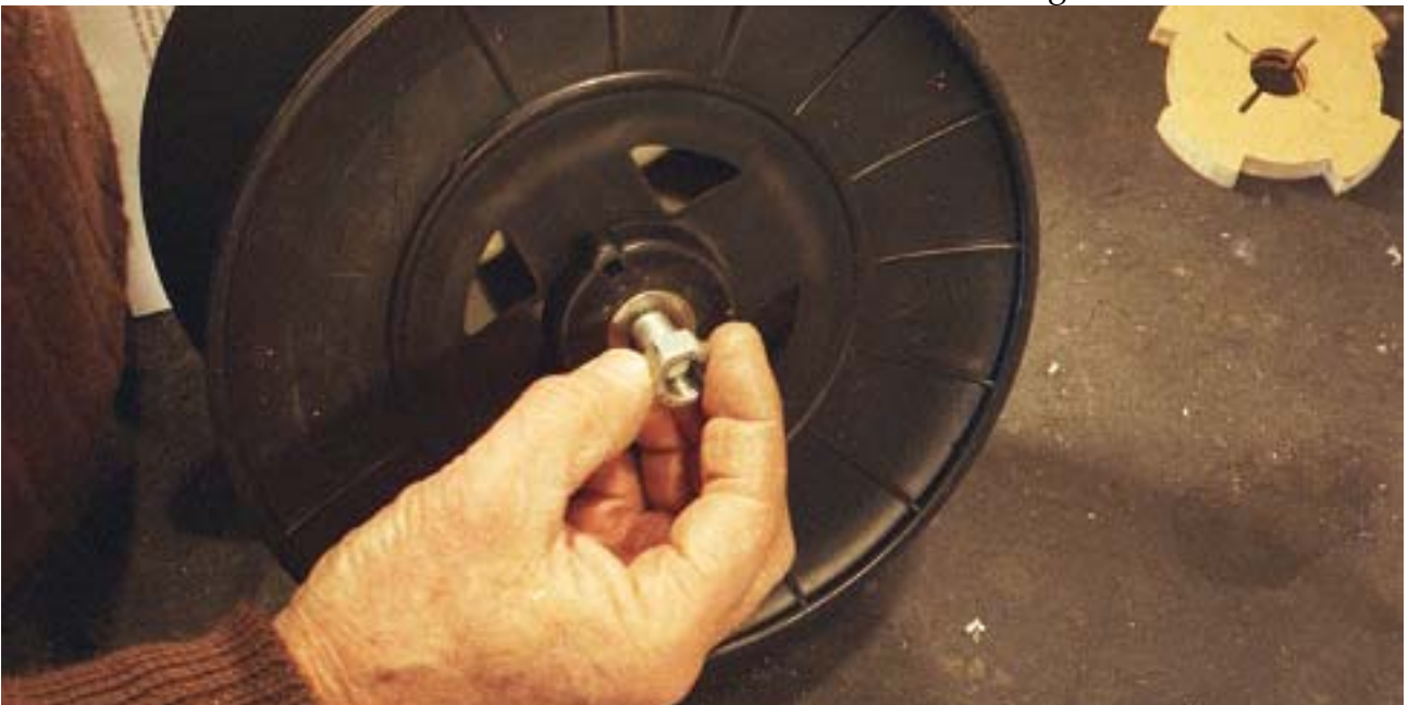
Figure 15. Attach washer and nut to handle bolt.
