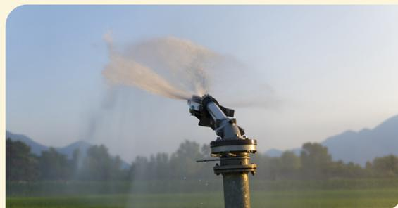
As you would expect for any hard-wearing mechanical equipment, irrigation performance checks on over 100 Hawke's Bay irrigation systems show that as irrigation systems age the performance deteriorates. This becomes more noticeable at about 10 years old. Conversely this study also showed that a well-maintained older system can still perform well.
