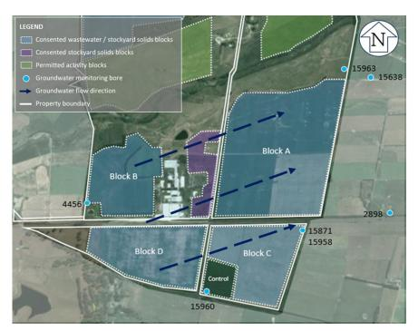
Figure 4.4.7.1(a): Groundwater monitoring bore locations.
