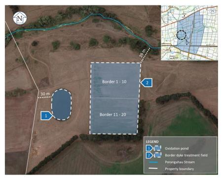
Figure 5.1.2: Indicative location of the domestic border dyke field and oxidation pond.
