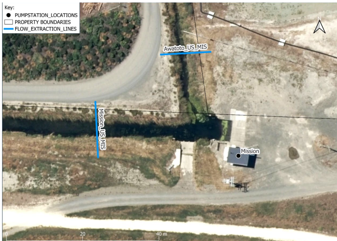
Figure 2. Flow Extraction Points for the Awatoto (Mission) Pump Station
