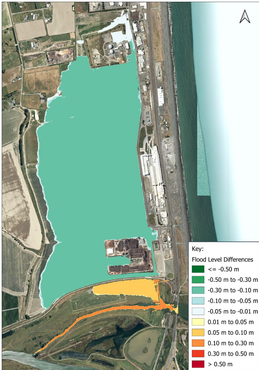
Figure 3. Flood Differences Between Existing and Upgraded Awatoto (Mission) Pump Station for 1% AEP RCP8.5 2081-2100 Event
