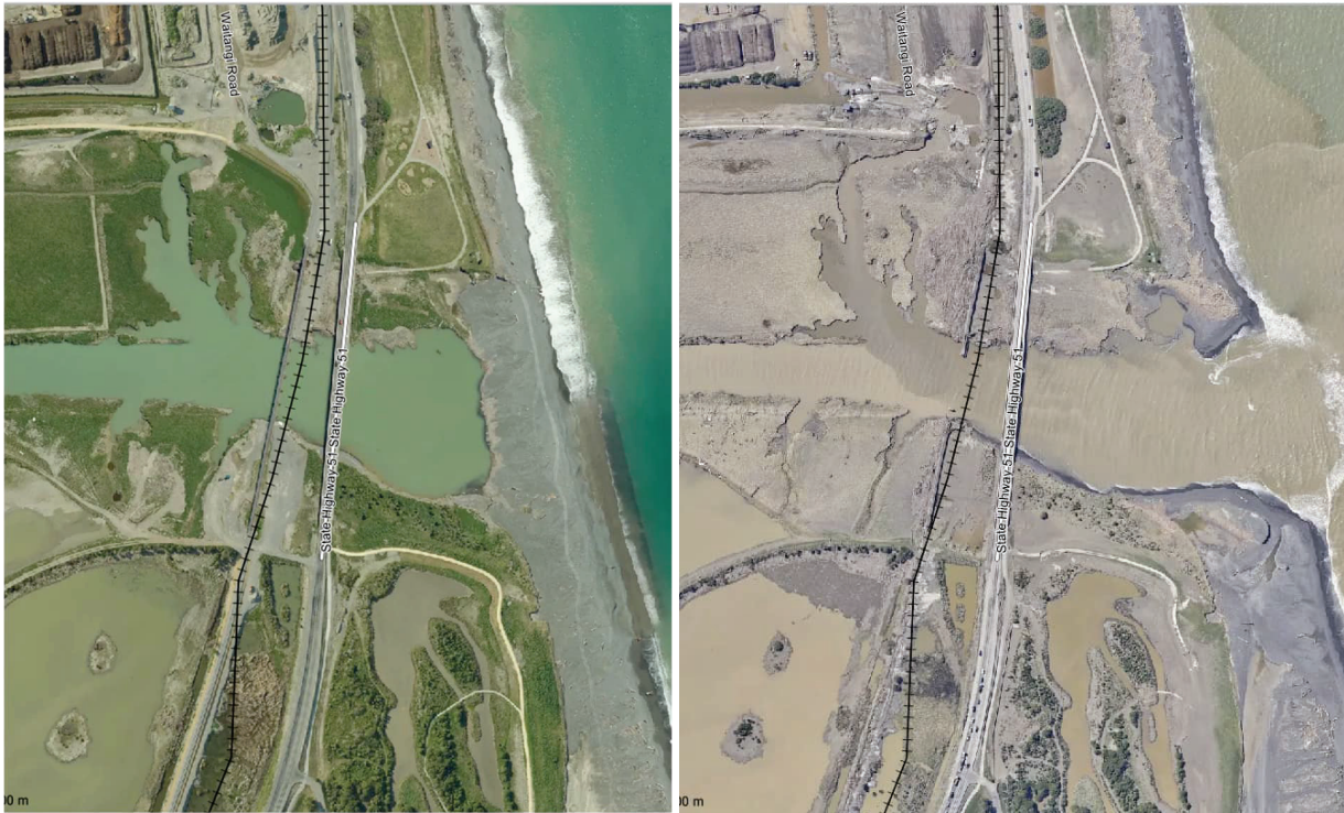
Figure 2. Closed mouth condition example (left) and post-cyclone mouth breached condition (right)
