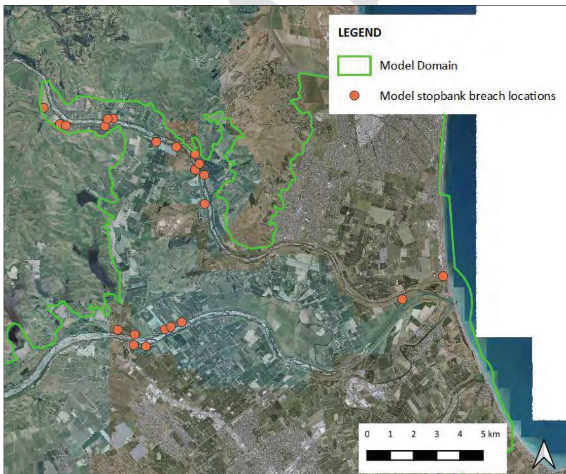
Figure 3.9: Stopbank breach locations applied to the model – Cyclone Gabrielle.
