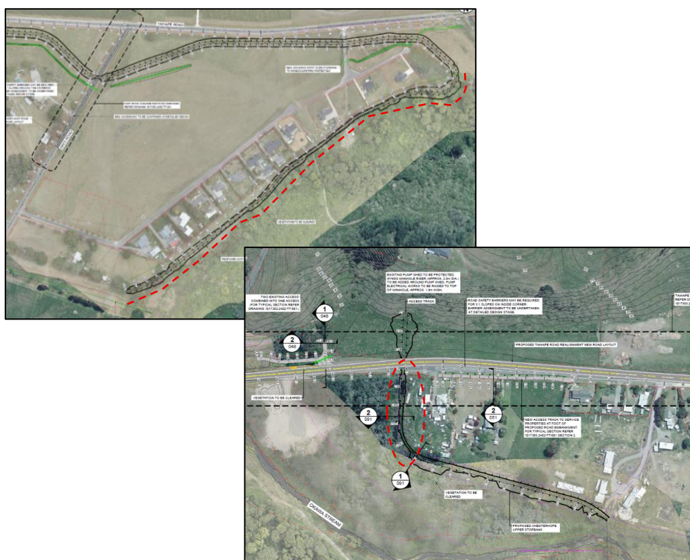
Figure 16: Areas of Vegetation Removal
