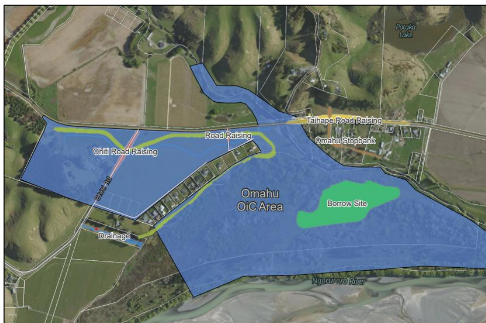
Figure 3: Flood Protection Works and OiC Footprint
