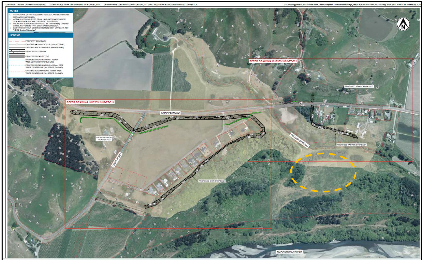
Figure 1: Proposed flood control measures for Taihape/ Ohiti Road area, orange dash indicates proposed quarry area (Source: HBRC, quarry site annotated in by AHB).
