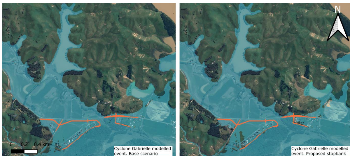
Figure 2.2: Estimated flood extent maps in modelled Cyclone Gabrielle event. Where flood depth is less than 50 mm, extent not shown.
