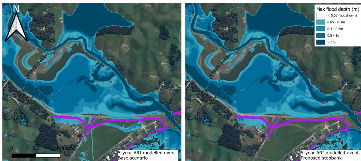
Figure 3.1: Estimated flood depth during the 5-year ARI event. Depths less than 50 mm not shown.
