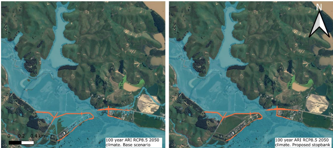
Figure 3-4 Modelled 100-year ARI flood extents with, and without, the proposed stopbank (Snip from Figure 2.1 T+T Effects Report)
