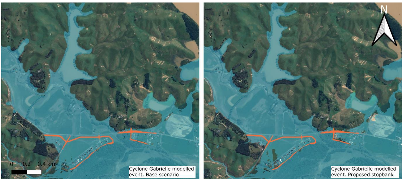
Figure 3-5 Modelled Cyclone Gabrielle flood extents with, and without, the proposed stopbank (Snip from Figure 2.2 T+T Effects Report)
