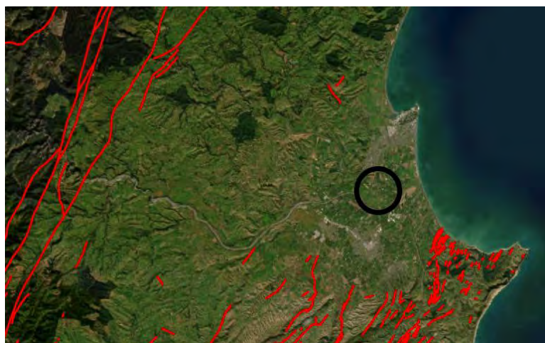
Figure 2.2: Active faults (faults indicated in red, general site location circled in black) 11 .
