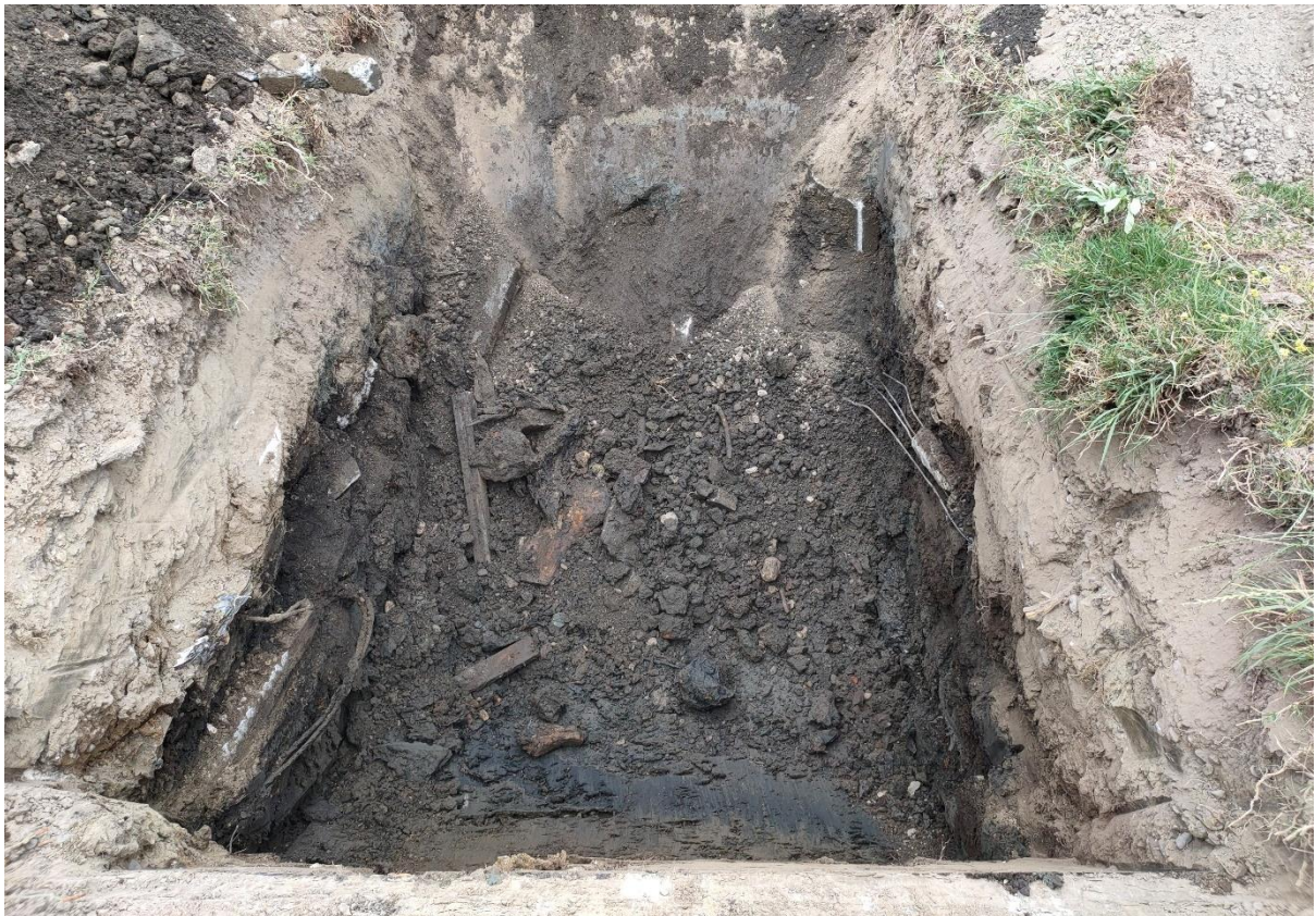
Photograph Appendix B.10: Site 3 – fill soils and refuse within S3_TP2.
