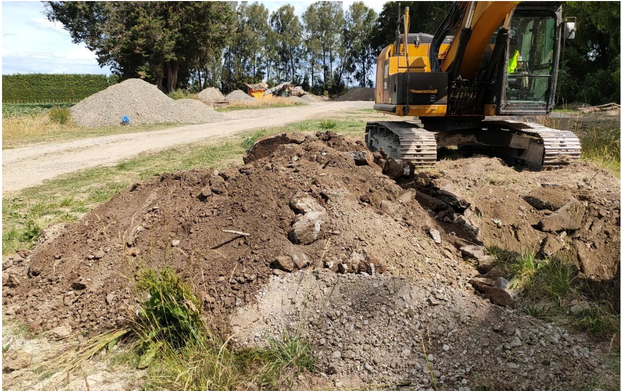
Photograph Appendix B.5: Site 2 – fill soils and concrete rubble in S2_TP4 and wider site. Facing south.
