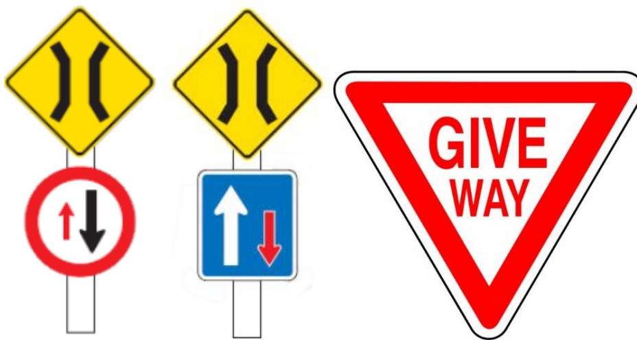
Figure 5.1: PW33 narrow bridge and RP52 single lane signage (left and centre), and RP2 give way sign (right).
