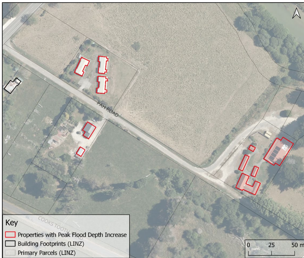
Figure 8. Pah Road building footprints that show an increase in peak flood depth as a result of the proposed flood mitigation works.
