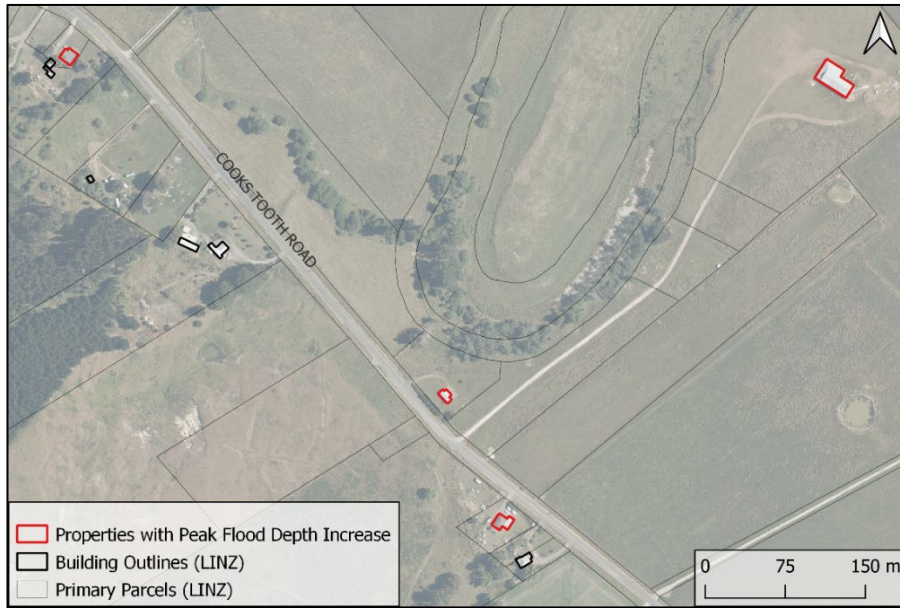
Figure 5. Cooks Tooth Road building footprints that show an increase in peak flood depth as a result of the proposed flood mitigation works.
