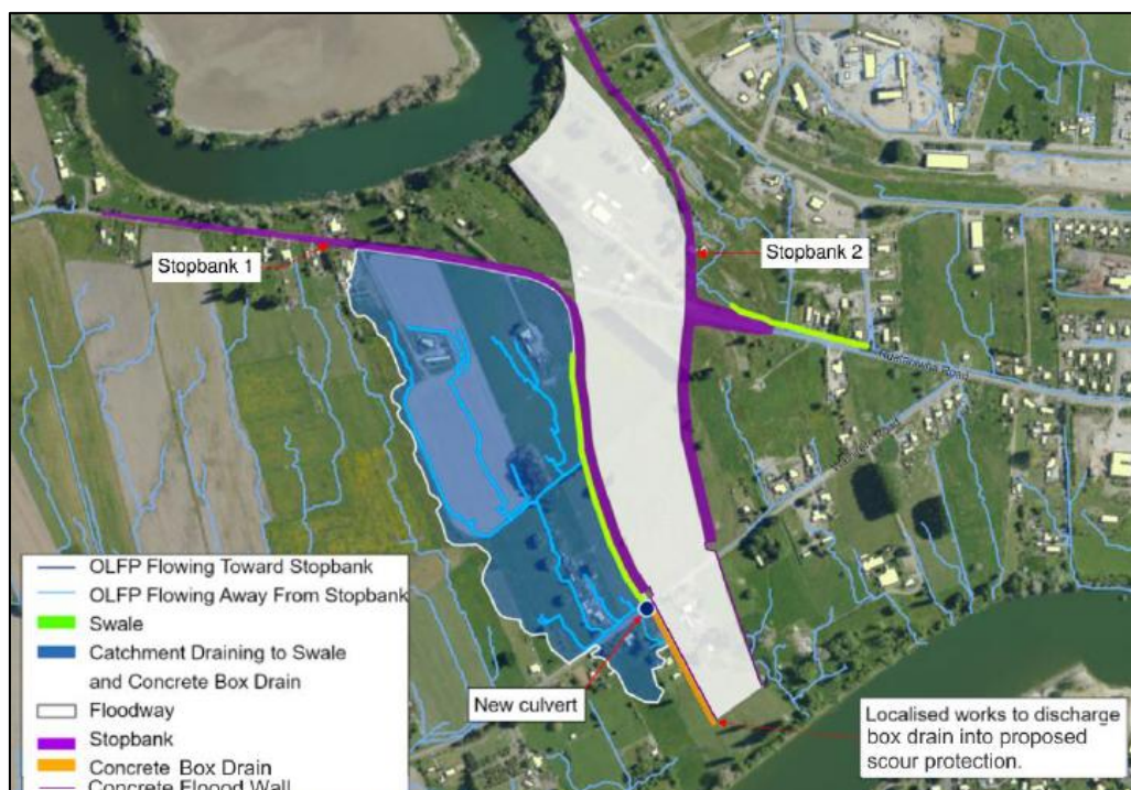
Figure 16: Cross Drainage Features
