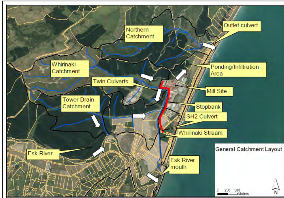
Figure 1: Existing Whirinaki flood control scheme
