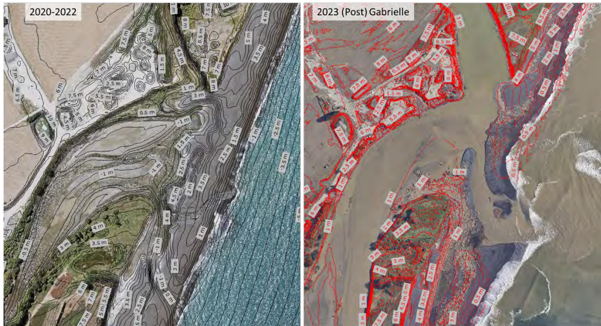
Figure 1-9: Comparison of aerial images and contours (NZVD2016) from 2020 and from the post Gabrielle survey in 2023
