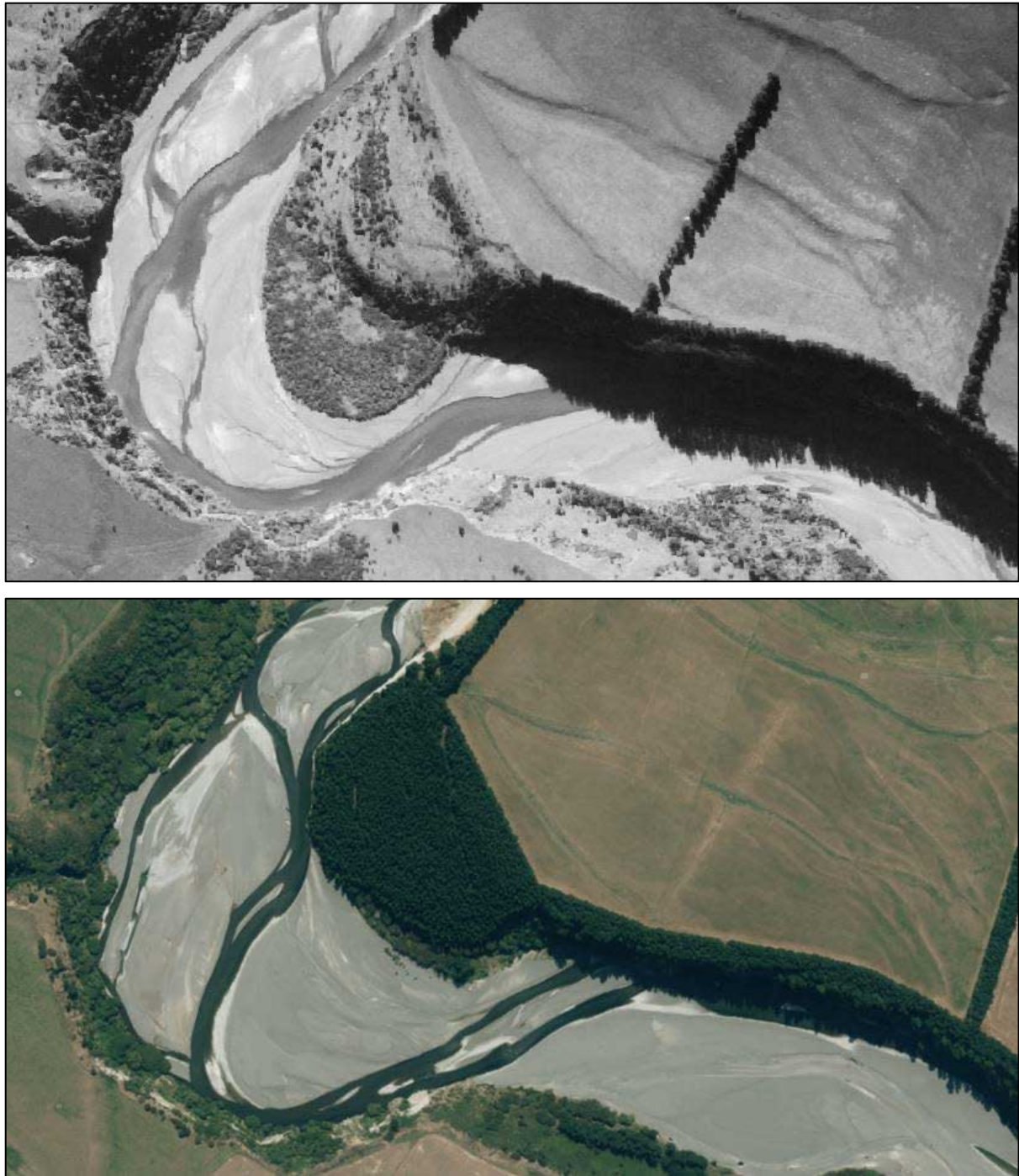
Figure 7: Aerial imagery 25 of the Ngaruroro River about 5km downstream from the Whanawhana Cableway in 1950 (top) and 2019/2020 (bottom). The width of the active channel remains similar (as per Figure 5).
