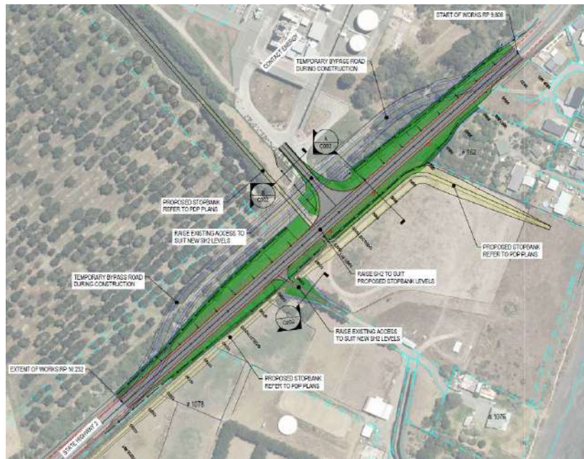
Figure 2 - SH2 Extent of Works
