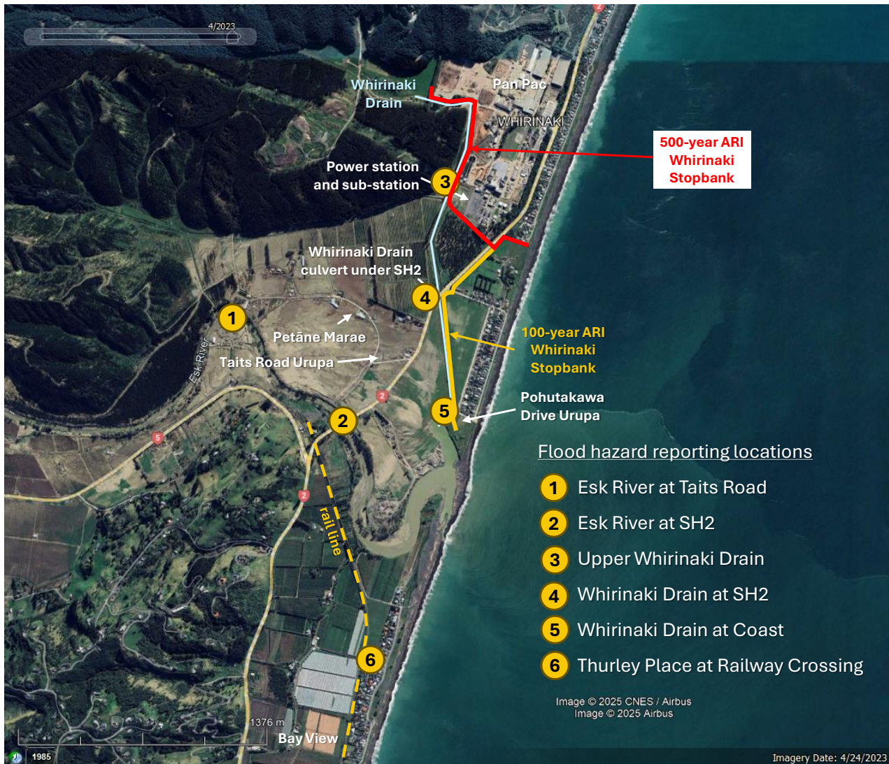
Figure 3-2 Flood hazard reporting locations
