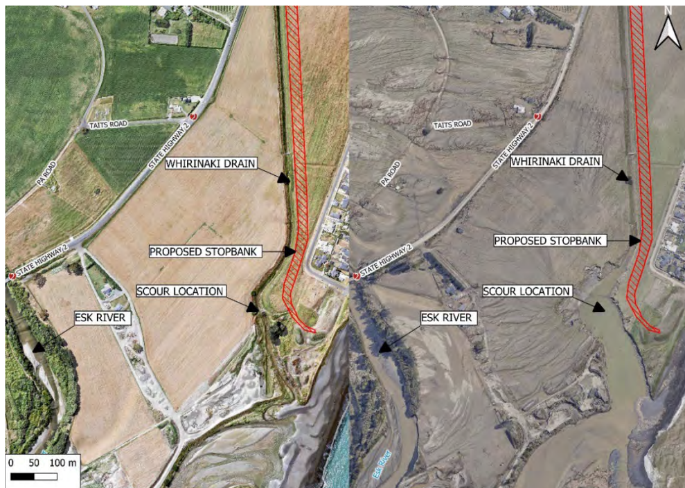
Figure 4: Pre (left- November 2021) and Post (right- April 2023) Cyclone Gabrielle comparison of lower Whirinaki Stream at confluence with Esk River (PDP, 2024)
