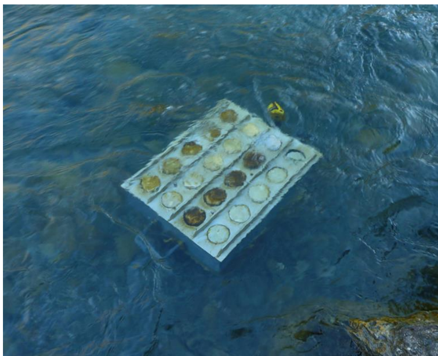
Figure 2-1: Nutrient diffusing substrate tray in the Ngaruroro River at Whanawhana. Five replicates of treatments from left to right: Nitrogen added, phosphorus added, nitrogen and phosphorus added and control without nutrient addition.
