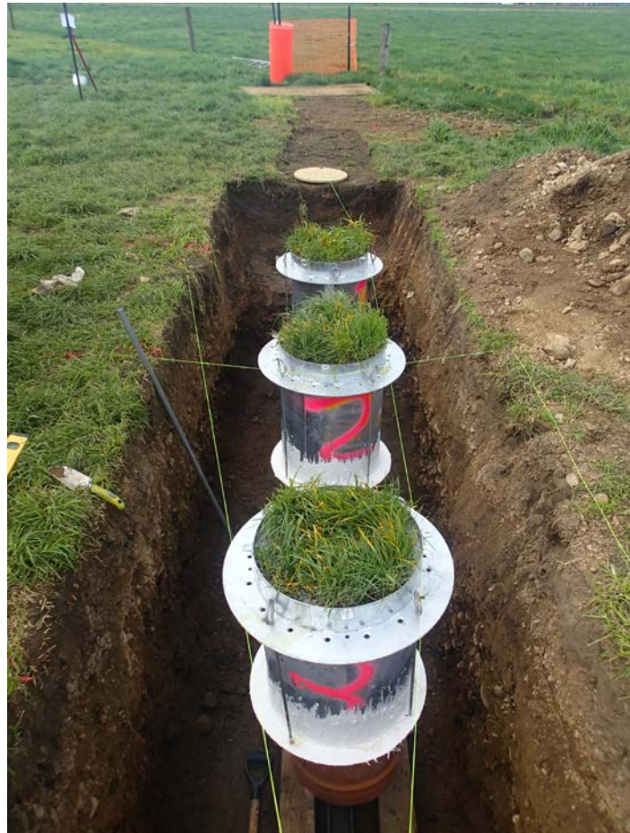
Figure 1: Lysimeters re-installed into the lysimeter pit and set to ground level. Lysimeter three is located in the foreground of the photograph, lysimeter two in the middle and lysimeter one furthest away.
