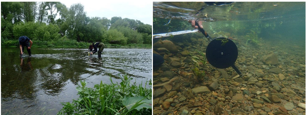
Figure 3-12: Hawke's Bay Regional Council staff measuring black disc sighting distance in the field.
