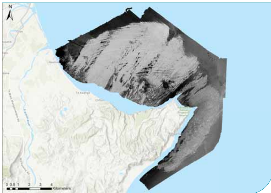
Figure 14-13. Backscatter images from the Multibeam surveys of Clive Hard. Light grey indicates areas of high reflectivity and hard substrate (eg, rocks, cobbles, and gravels). Dark grey areas have low reflectivity and soft substrate.
