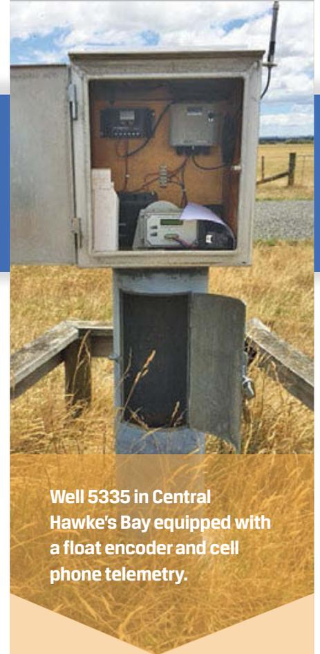
**Well 5335 in Central Hawke's Bay equipped with a float encoder and cell phone telemetry.**
