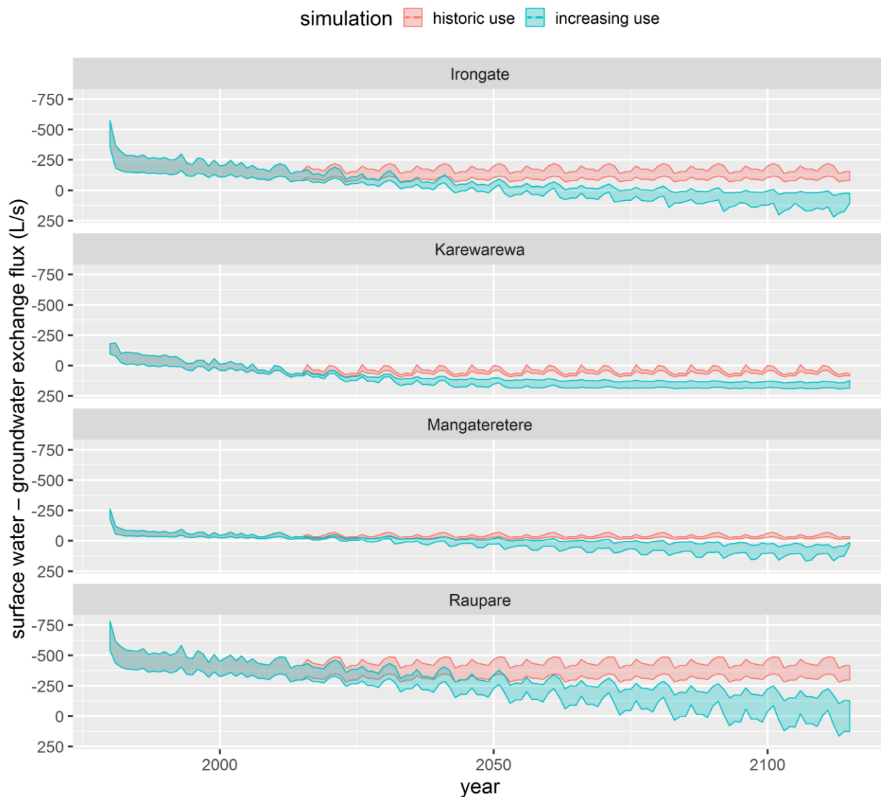
Figure 6-16: Surface water - groundwater exchange flux for all realisation for 100 years simulation for small springs. Showing "historical use" and "increasing use" simulations. Dashed line represents original prediction. Shading represents 5th and 95th percentile of predictions.
