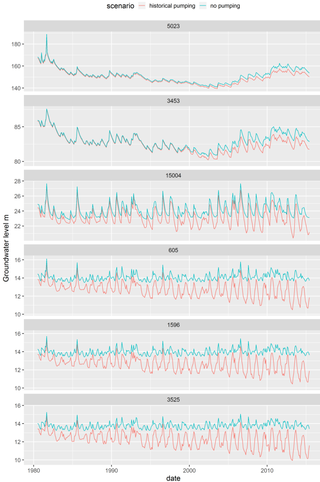
Figure 3-22: Hydrographs of simulated groundwater levels (masl) in Heretaunga Aquifer. Set 3 of bores identified in Figure 3-19 (Kikowhero-Maraekakaho - Bridge Pa - Pakipaki). Note that bores 5023 and 3453 show a greater range of groundwater levels
