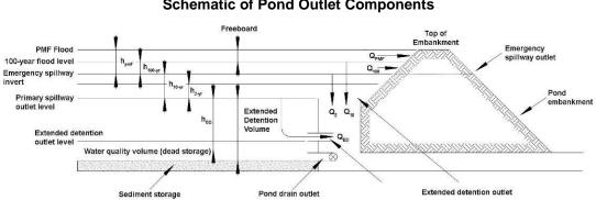
Figure 7-18 Schematic of Pond Outlet Components
