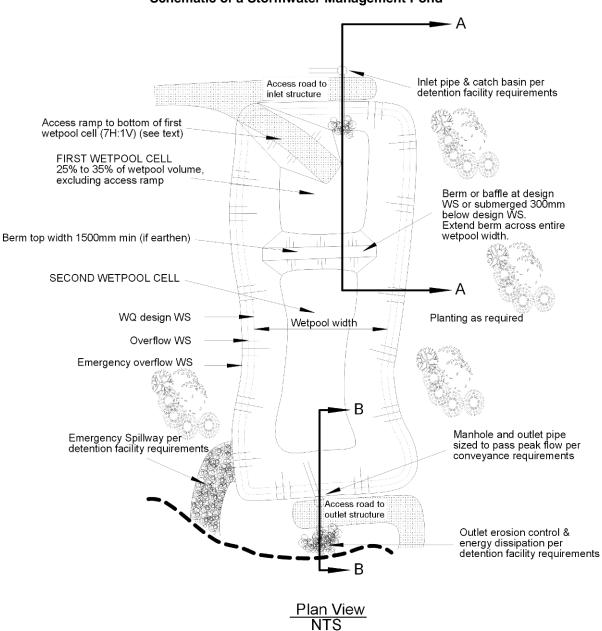
Figure 7-16 Schematic of a Stormwater Management Pond
