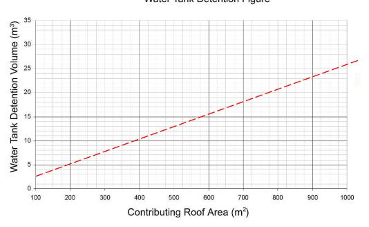
Figure 7-28 Water Tank Detention Figure
