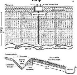
2. Once the peak discharge is determined, that discharge can be entered into Manning's equation to determine the width of the filter strip.
