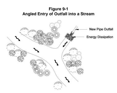
The impact of new pipe outfalls can be significantly reduced on receiving streams by locating them further back from the stream edge and digging a channel from the outfall to the stream. This would allow for energy dissipation before flows enter the stream, as shown in Figure 9-1. At a minimum, the pipe outfall should be located far enough back from the stream edge to prevent the energy dissipater intruding on the channel.
