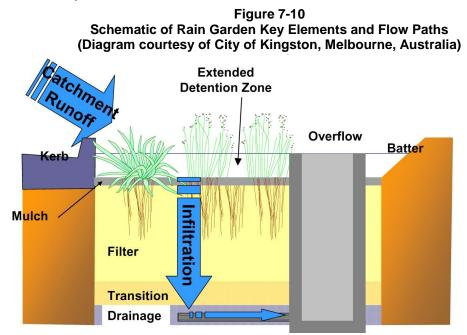
Rain garden design, as shown in Figure 7-10 differs only slightly from sand filter design. Where sand filtration relies on water quality treatment via passage of stormwater through sand, rain gardens incorporate plants and soils for removal of contaminants. A downside of the use of plants and soils rather than sand is a reduction in the permeability rate. This results in rain gardens being larger in surface area than sand filters.
