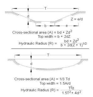
8. Use Manning's equation for calculating dimensions of the swale by using first approximations for the hydraulic radius and dimensions for selected shape.
