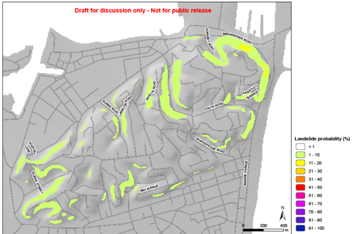
Figure 4.5 EIL probability class colour map of Bluff Hill, Hawke's Bay based on a 0.64 g PGA at a return period of 2500 years.
