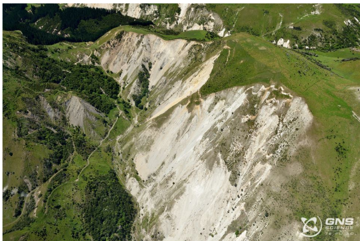
Figure 1.4 Soil slope deformation associated with the Kekerengu Fault near the junction to Clarence River following the 2016 Kaikōura Earthquake.
