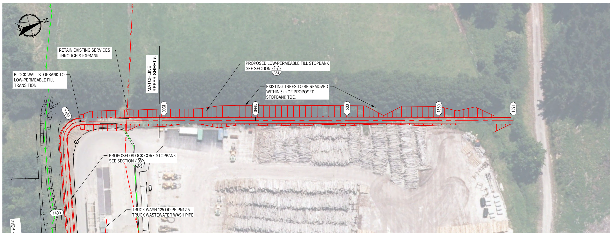
PROPOSED STOPBANK PLAN CH.1500 TO CH 1693 SCALE 1:1000
