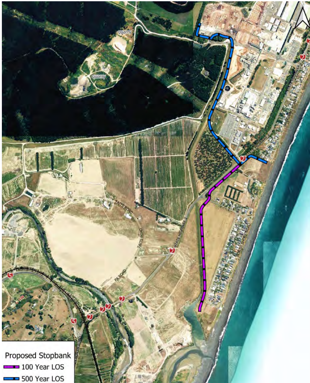
Figure A1: Proposed Whirinaki stopbank layout.
